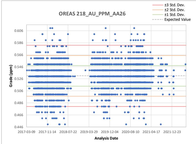
Figure 11-9: Results of standard OREAS 218 using AA26 Method
