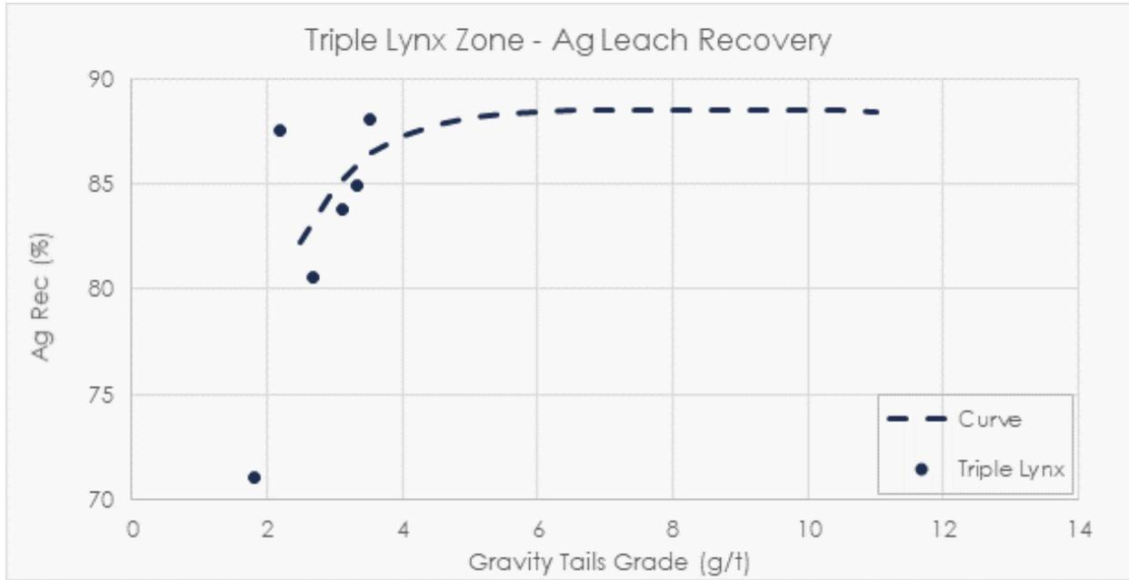
Figure 13-44: Triple Lynx zone silver recovery curve
