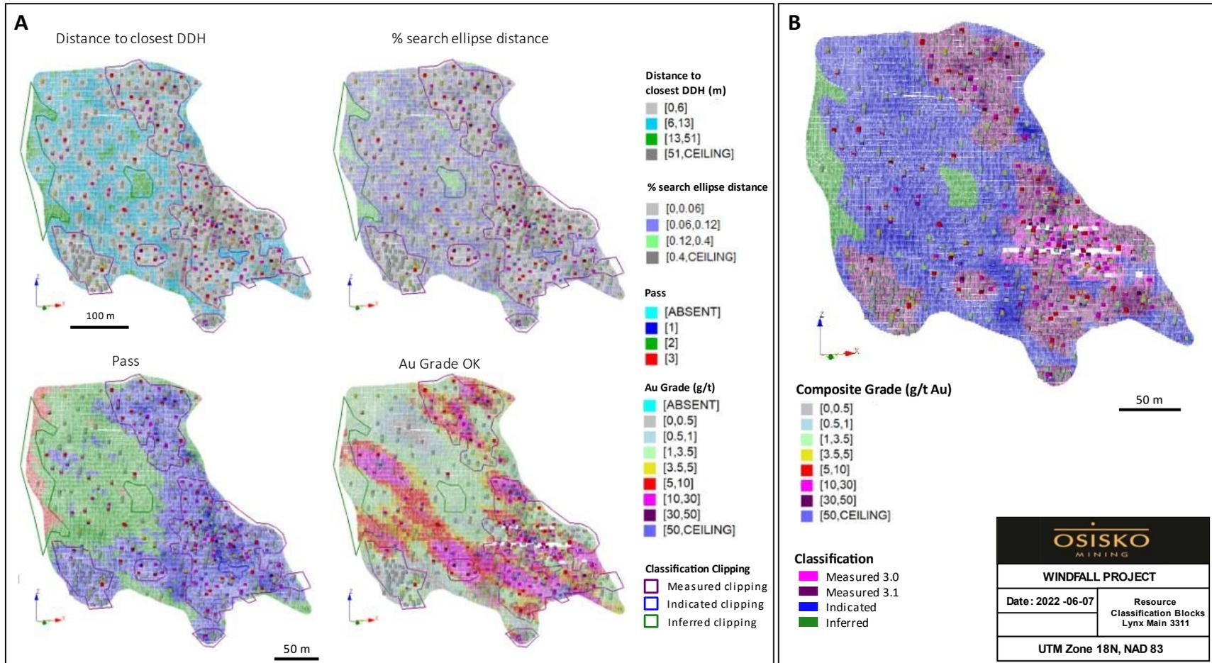
Figure 14-14: Example of resource classification for blocks in lens 3311 in Lynx Main zone
