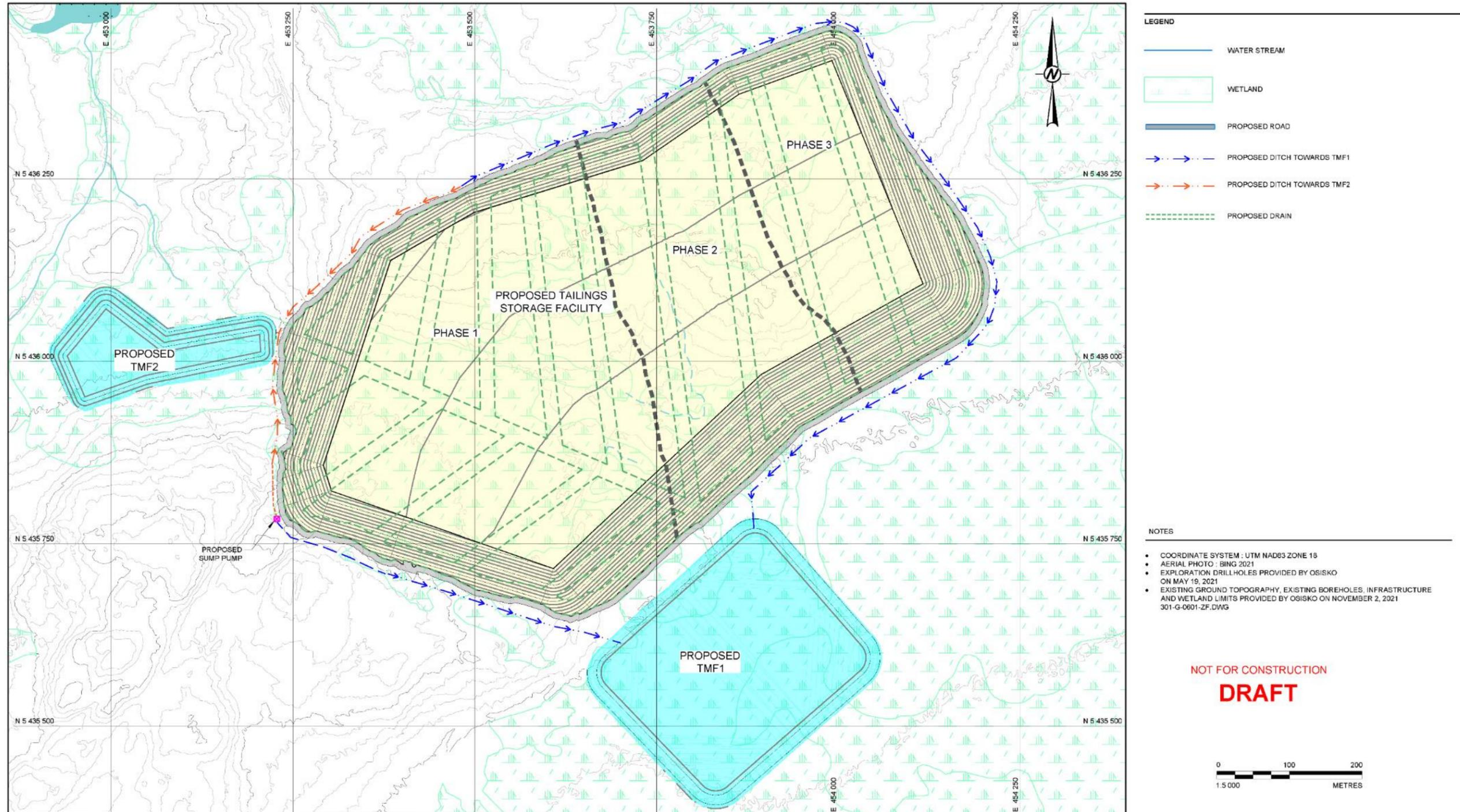
Figure 18-16: Plan view of the tailings management facility
