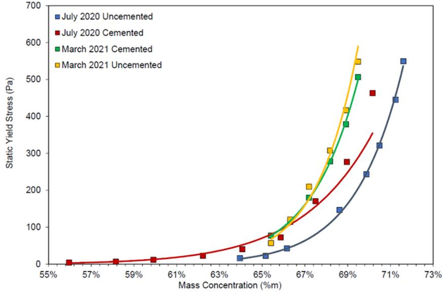
Figure 13-8: Static yield stress vs. mass concentration
