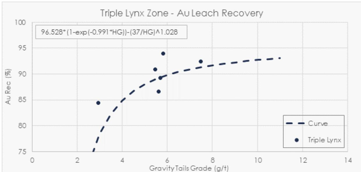
Figure 13-39: Triple Lynx zone gold recovery curve
