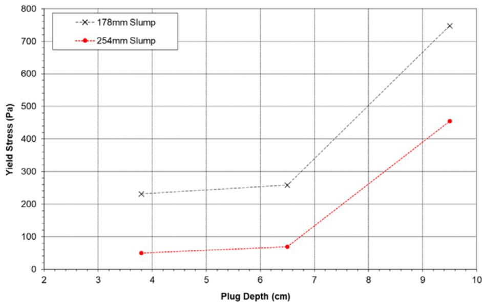
Figure 13-22: Plug yield stress for Tailings 37 µm sample
