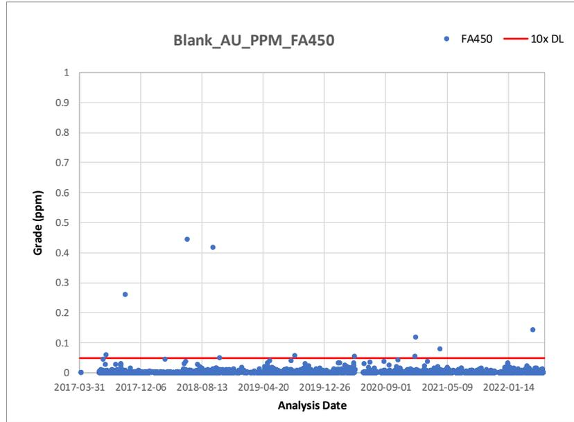
**Figure 11-3: Time series plot for blank samples assayed by Bureau Veritas (FA450 Method)**
