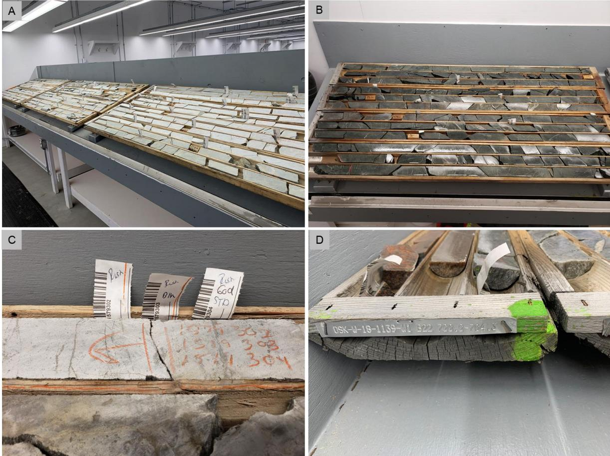
Figure 12-4: A) and B) Core review in the core logging facility, with C) Sample tags; and D) Identification tags
