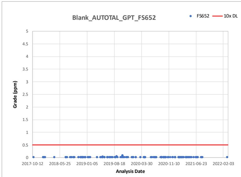
Figure 11-6: Time series plot for blank samples assayed by Bureau Veritas (FS652 Method)
