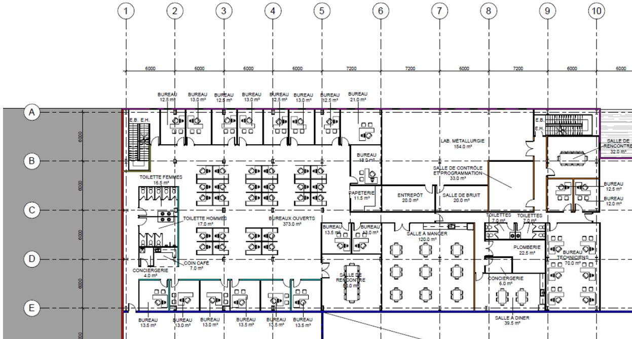
Figure 18-11: Plan view of 1<sup>st</sup> floor office
