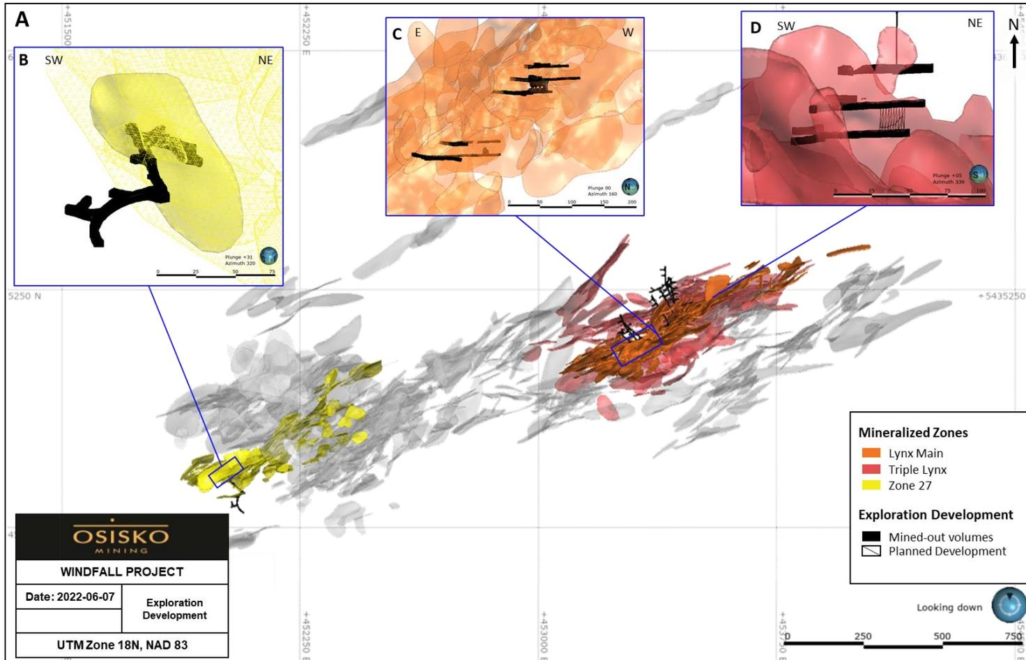
Figure 14-6: Exploration ramp intersecting mineralization of the Windfall deposit
