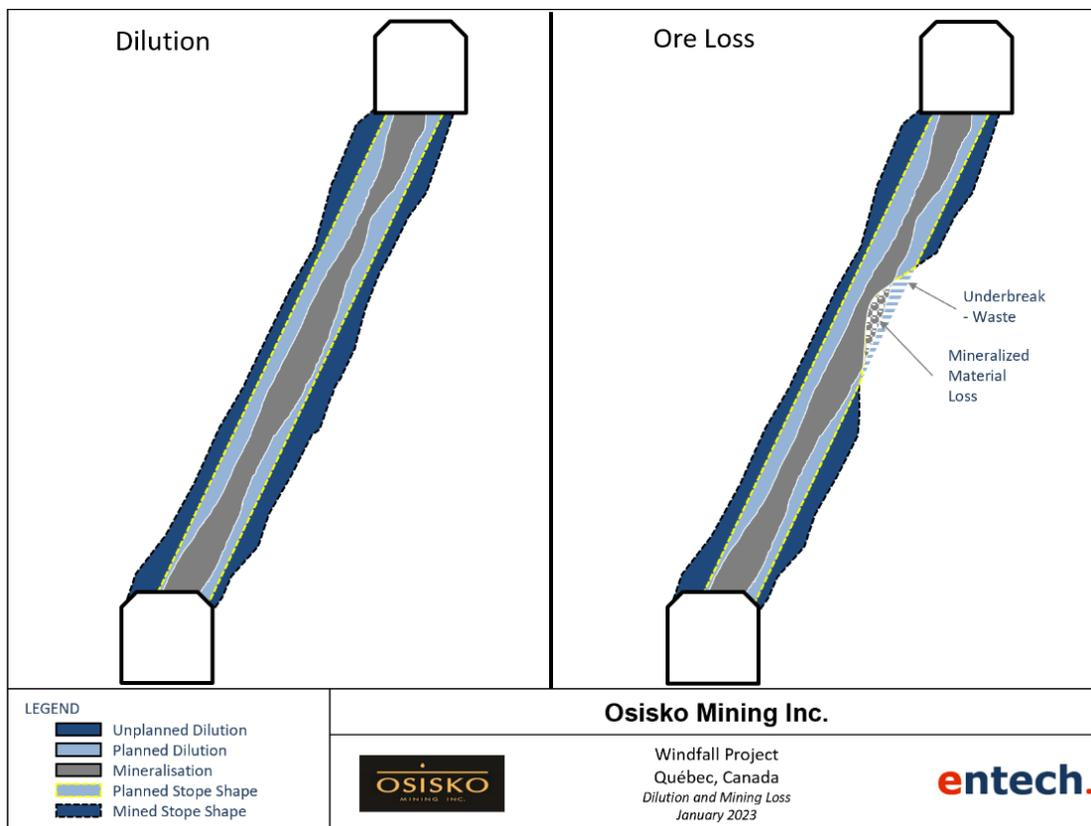
Figure 16-2: Dilution and mining recovery
