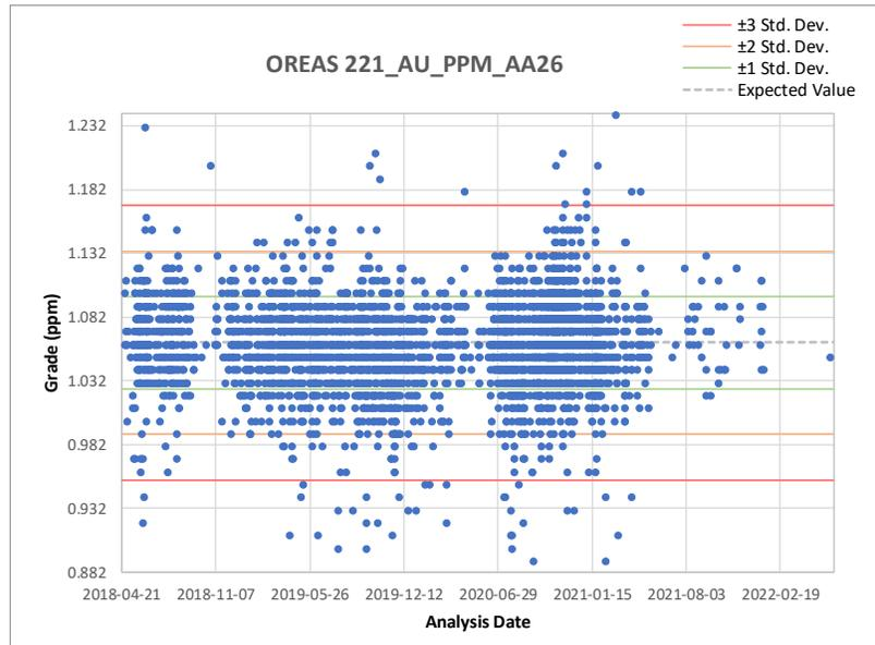
Figure 11-10: Results of standard OREAS 221 using AA26 Method
