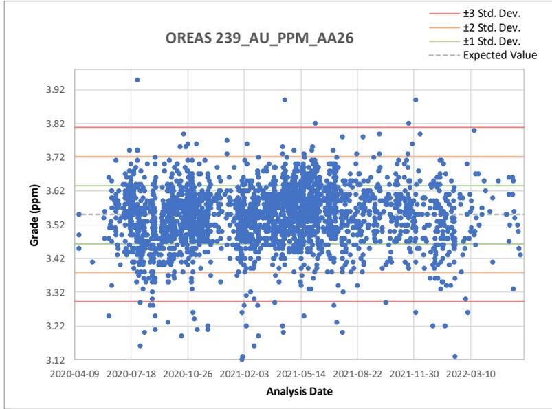
Figure 11-11: Results of standard OREAS 239 using AA26 Method
