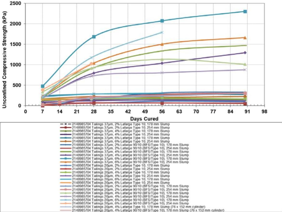
Figure 13-28: UCS results for samples Tailings 37 and 20 µm
