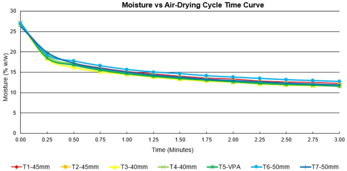
Figure 13-33: Drying time effect on cake moisture
