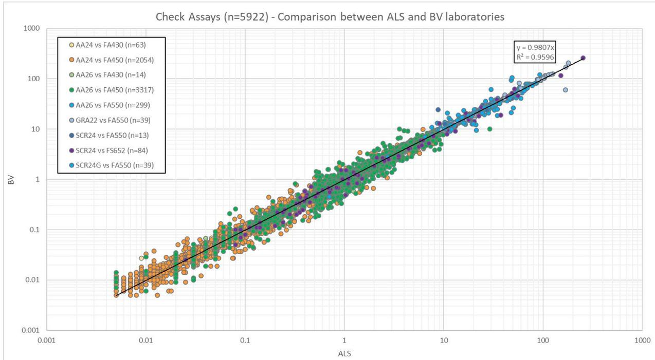
**Figure 11-13: Post 2014 mineral resource estimate laboratory pulp duplicates for gold (g/t)**
