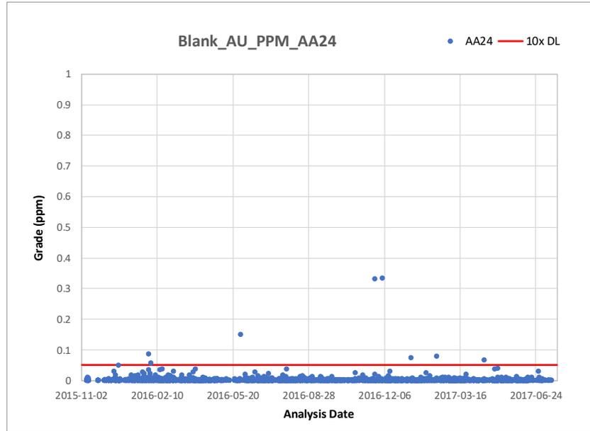
**Figure 11-1: Time series plot for blank samples assayed by ALS (AA24 Method)**
