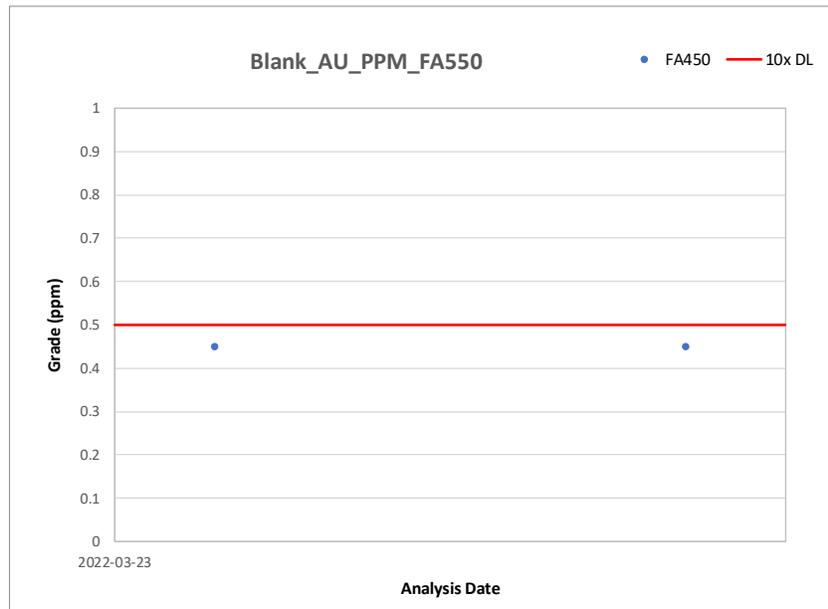
**Figure 11-4: Time series plot for blank samples assayed by Bureau Veritas (FA550 Method)**
