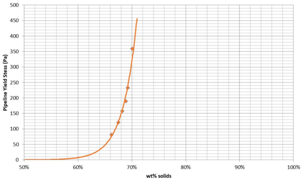
Figure 13-26: Pipeline yield stress vs. wt% solids
