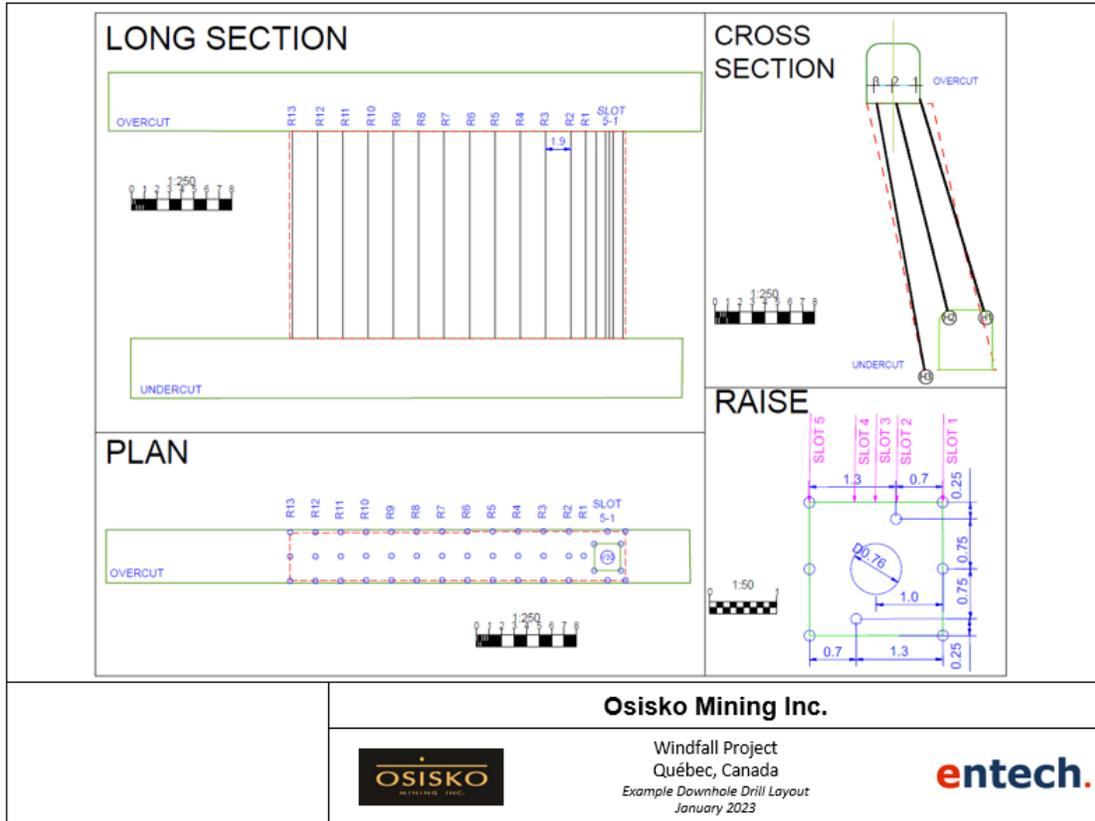
Figure 16-13: General arrangement for downhole stope design
