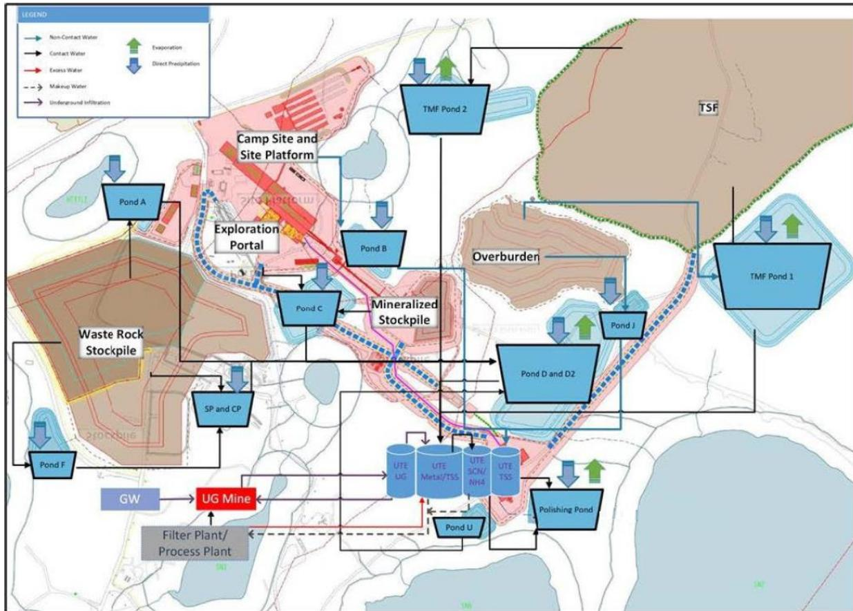
Figure 20-4: Water balance conceptual flow diagram – Phase 2
