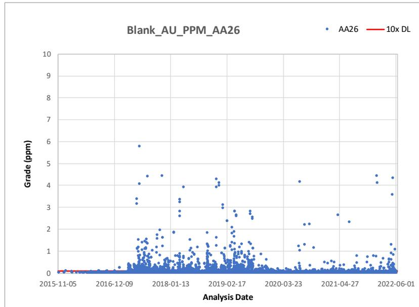
**Figure 11-2: Time series plot for blank samples assayed by ALS (AA26 Method)**
