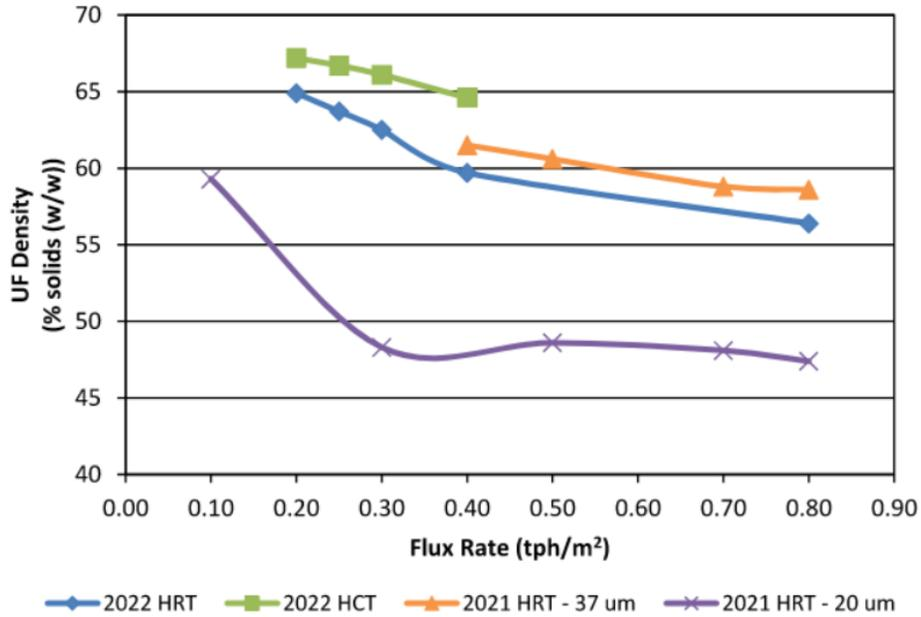
Figure 13-30: Historical underflow solids content comparison for different P<sub>80</sub>
