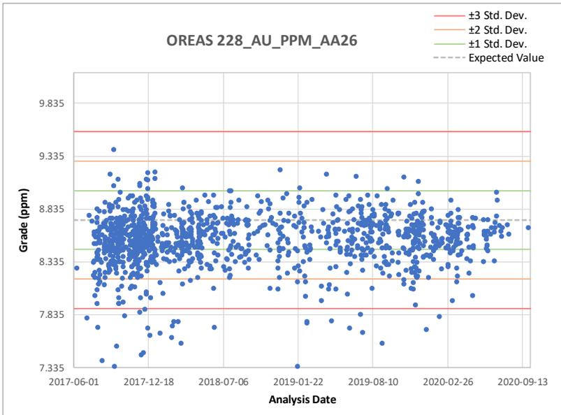
Figure 11-12: Results of standard OREAS 228 using AA26 Method
