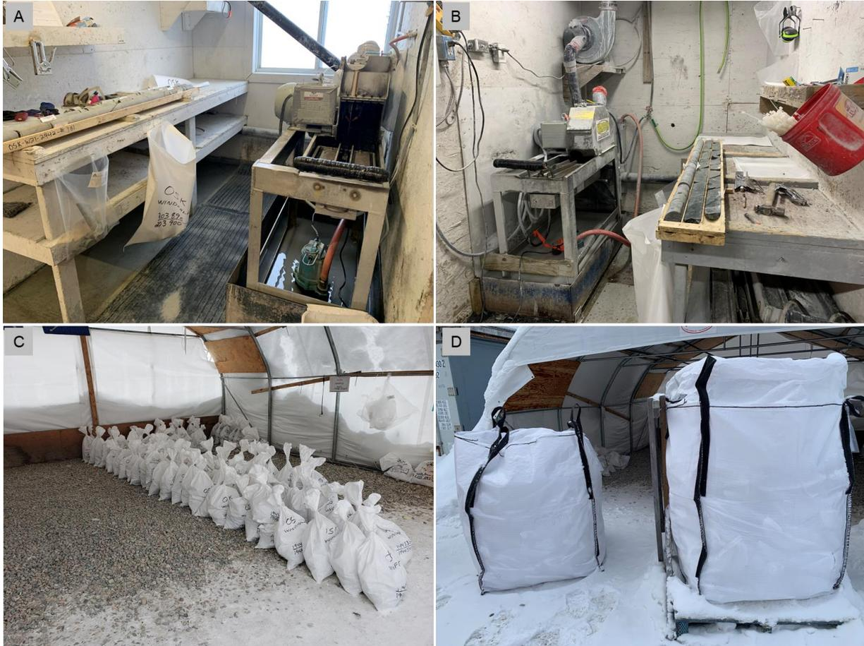
Figure 12-3: A) and B) Sample preparation room; C) and D) Samples ready for shipment to the laboratory
