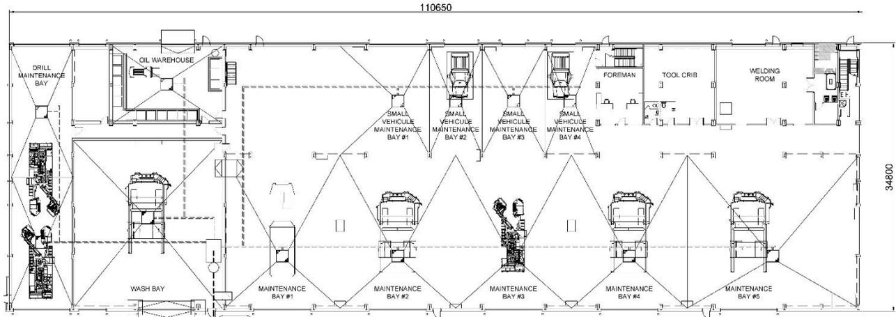
Figure 18-7: Truck shop layout (first floor)
