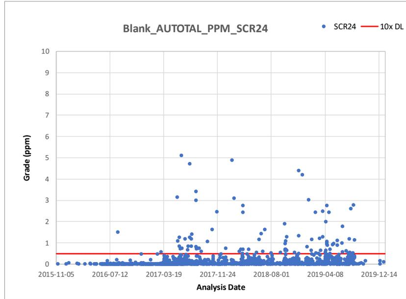
**Figure 11-7: Time series plot for blank samples assayed by ALS (SCR24 Method)**
