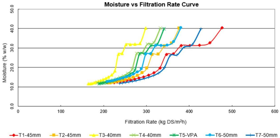
Figure 13-34: Filtration rate vs. cake moisture
