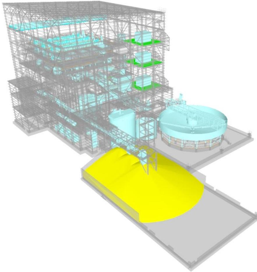
**Figure 18-13: Tailings filtration and paste backfill plant layout**
