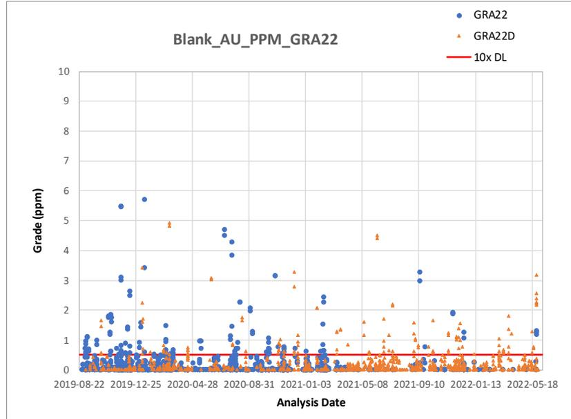
Figure 11-5: Time series plot for blank samples assayed by ALS (GRA22 Method)
