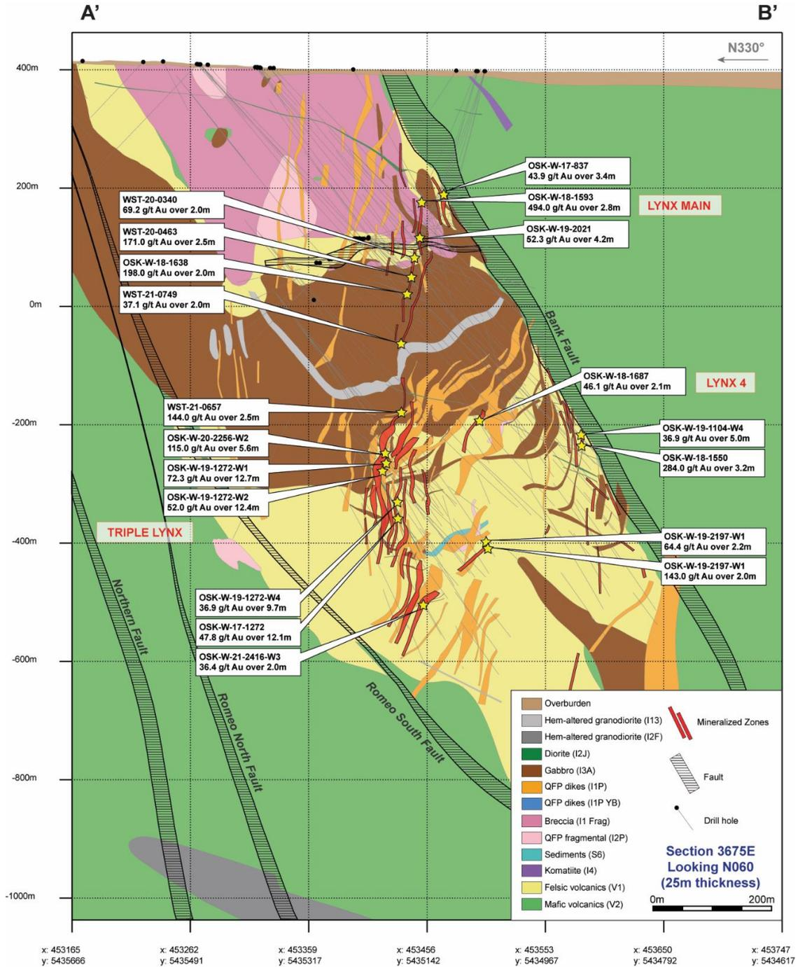
Figure 7-9: Simplified northwest-southeast vertical cross-section of the geology of the Lynx area of the Windfall deposit
