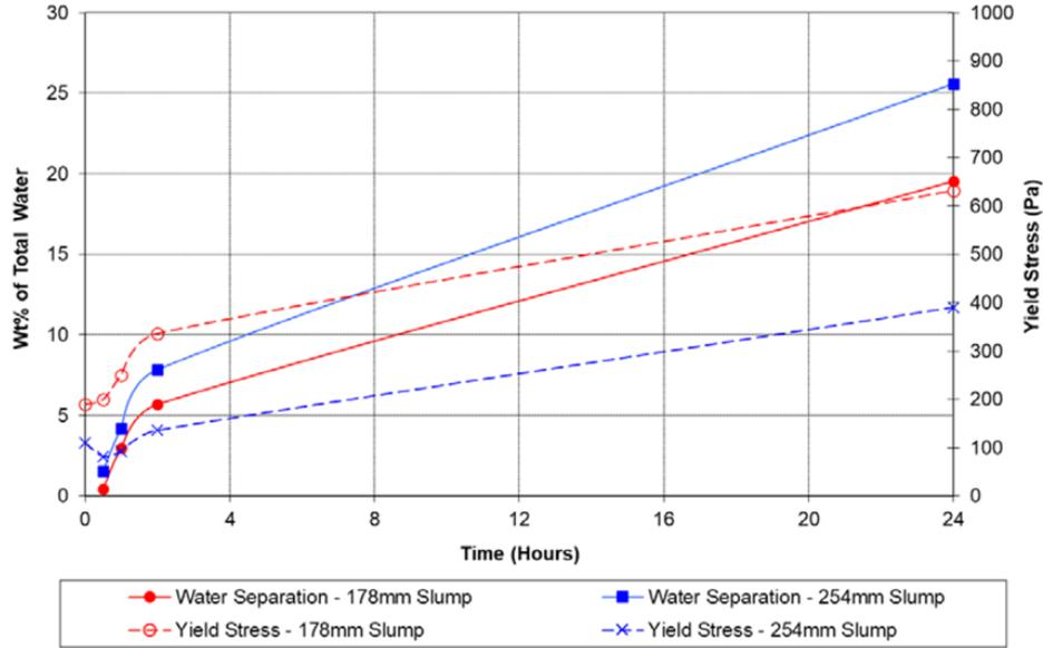
Figure 13-21: Water bleed and yield stress vs. time for Tailings 37 µm sample
