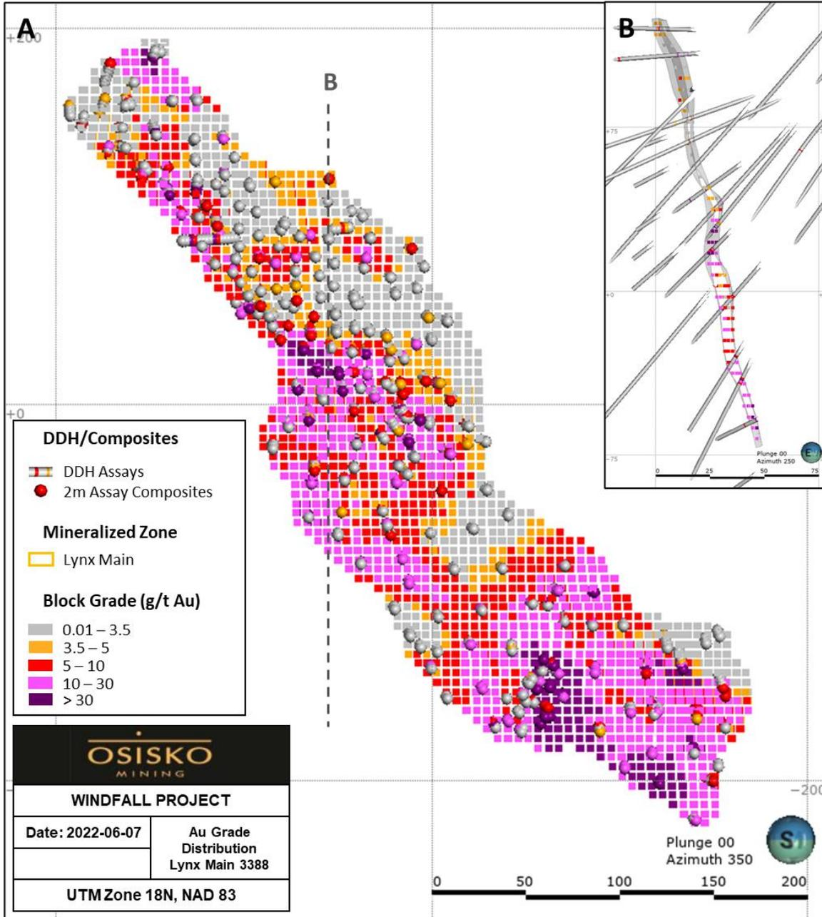
Figure 14-11: Gold grade distribution in mineralized lens 3388, Lynx Main zone
