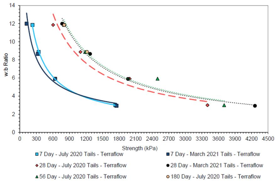
Figure 13-18: Water-to-binder ratio curves with "TerraFlow" binder
