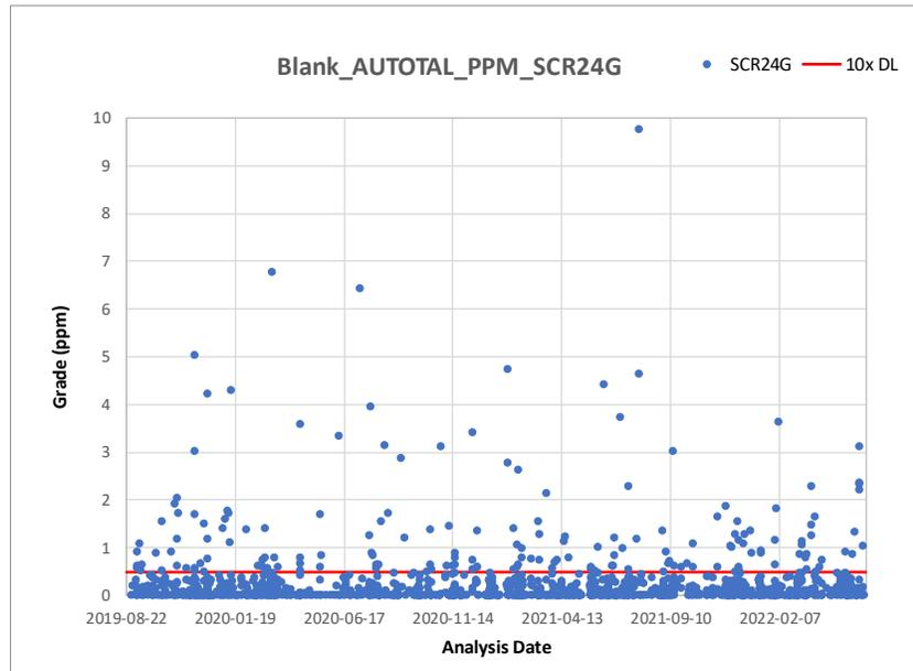
**Figure 11-8: Time series plot for blank samples assayed by ALS (SCR24G Method)**
