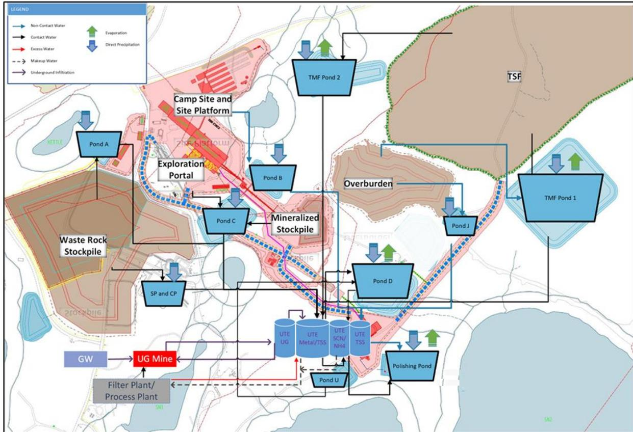
Figure 20-3: Water balance conceptual flow diagram – Phase 1
