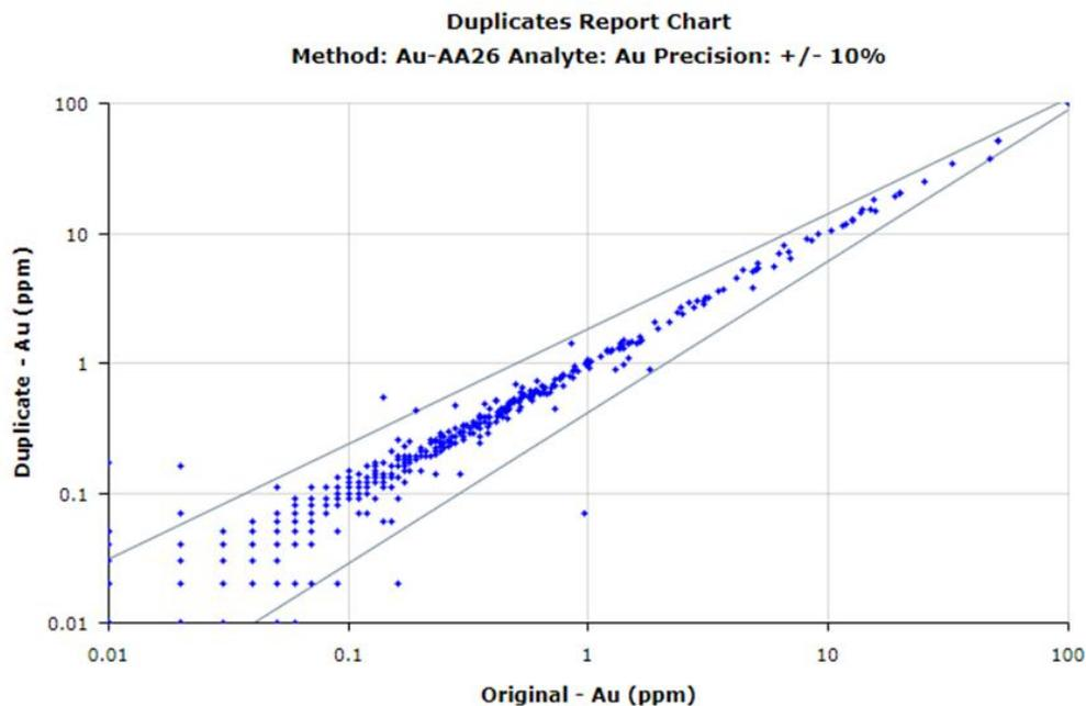
Figure 11-15: ALS pulp duplicates for Windfall samples (AA26)
