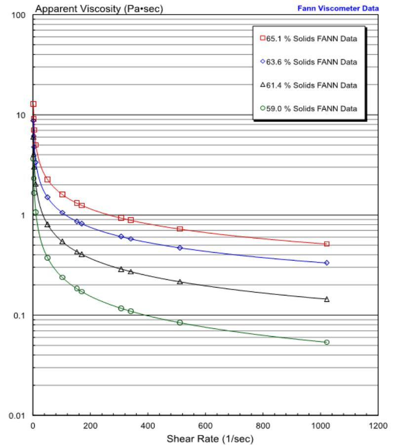
Figure 13-6: Apparent viscosity vs. shear rate
