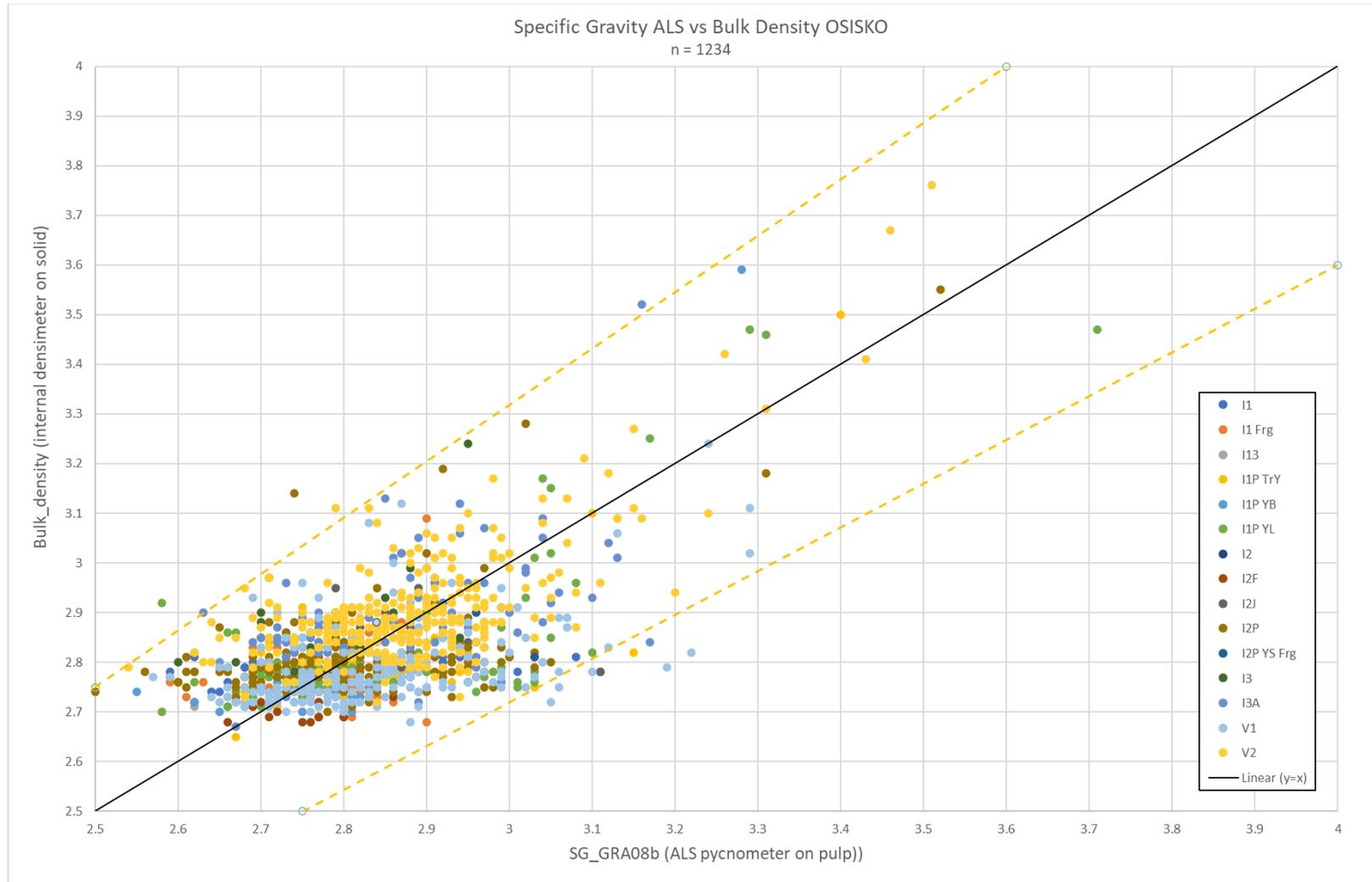
Figure 11-14: Laboratory specific gravity (GRA08b) and internal bulk density measurement correlation (Eagle Hill and Osisko)
