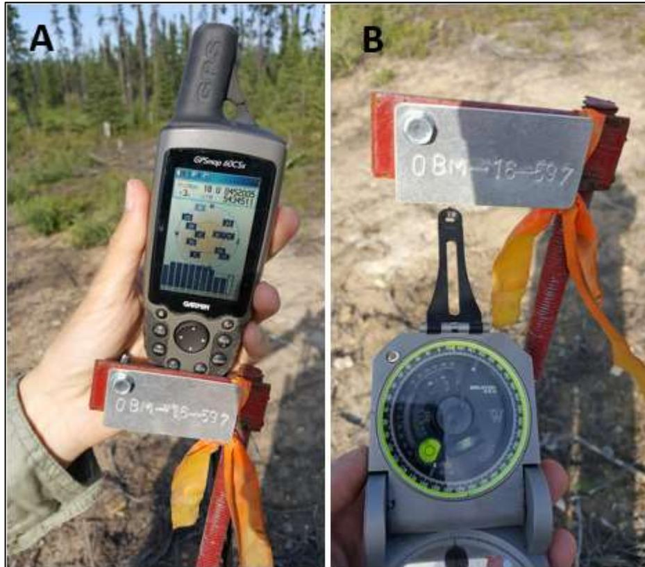
**Figure 12-3: A) Photograph showing the GPSMAP 60CSx used to verify the location of a drill collar during the site visit – Hole OBM-16-597. B) Photograph showing one of the metal identification labels used for most drill hole collars on the Windfall Lake Project – Hole OBM-16-597.**
