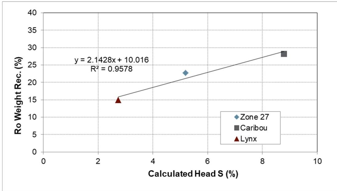
Figure 13-6: Rougher weight recovery vs. %S in feed
