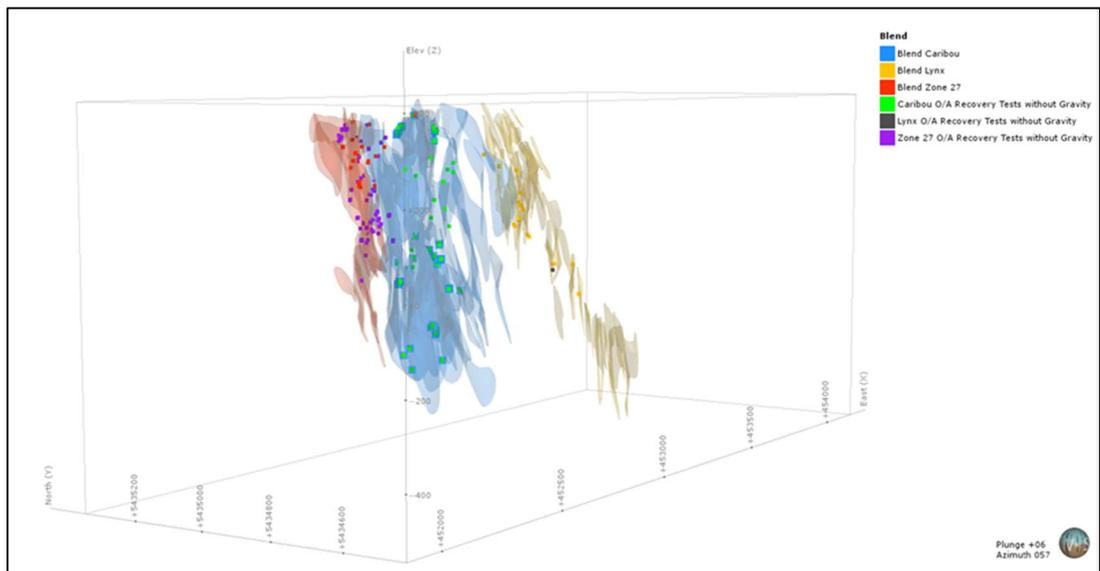
**Figure 13-4: Looking N050 view of recovery samples holes locations**
