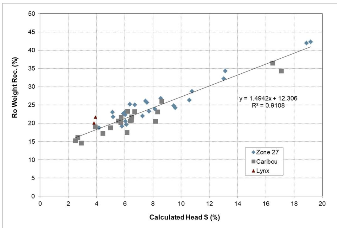
Figure 13-8: Rougher weight recovery vs. %S in feed
