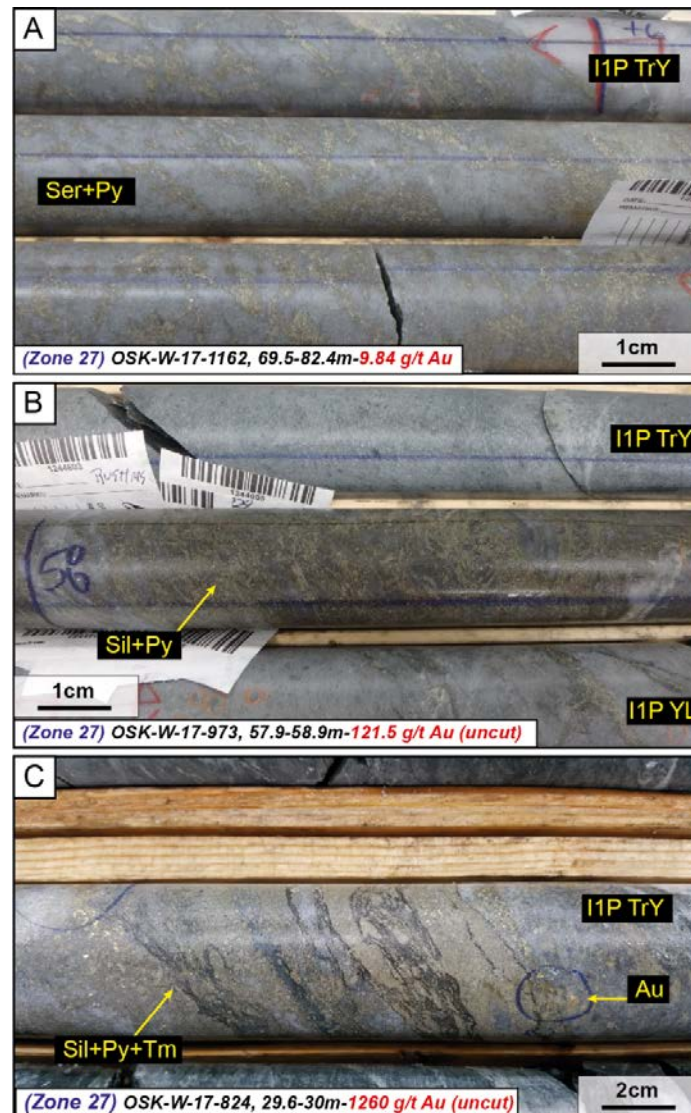
Figure 7-11: Typical mineralization and associated alteration styles in Zone 27 of the Windfall Lake deposit. A) Pyrite stringers associated with strong phyllic alteration within a quartz-feldspar porphyry dike (I1P TrY). B) Strong silica alteration associated with gold-bearing pyrite mineralization at the contact between two phases of quartz-feldspar porphyry dikes. C) Visible gold associated with abundant pyrite and tourmaline mineralization in a strongly silica-sericite altered quartz-feldspar porphyry dike. All gold grades (Au g/t) are cut to 100 g/t unless indicated.
