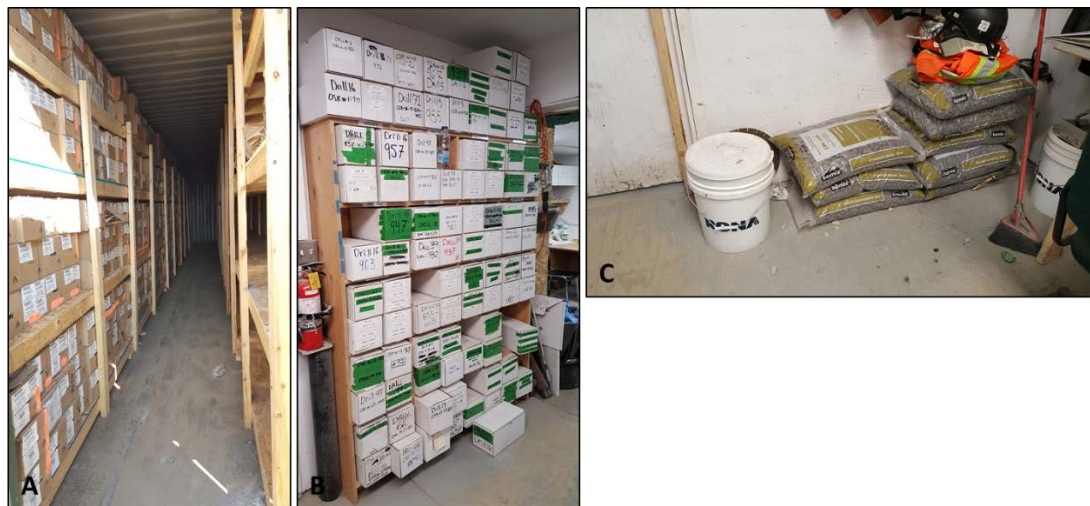
Figure 12-2: A) Photograph of boxes containing pulps; B) Boxes containing standards used during the drilling programs; C) Commercial crushed stones used as blank material during the drilling programs.
